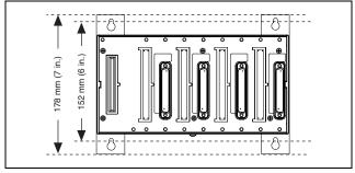
Figure 13. Dimensions of Compact FieldPoint Vertical Panel-Mount Kit
